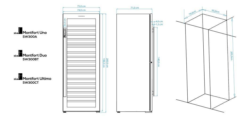
This model is design for free-standing installation. Built-in installation is possible if the wine cooler has at least 5cm space on each side (like the above drawing). The air should be able to move freely in the space around the wine cooler.
