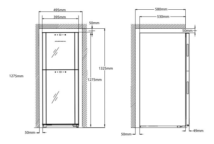
This model is designed for free-standing installation. Built-in installation is possible if the wine cooler has at least 5cm space on each side (like the above drawing). The air should be able to move freely in the space around the wine cooler.
