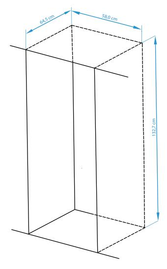
This model is designed for free-standing installation. Built-in installation is possible if the wine cooler has at least 5cm space on each side (like the above drawing). The air should be able to move freely in the space around the wine cooler.
