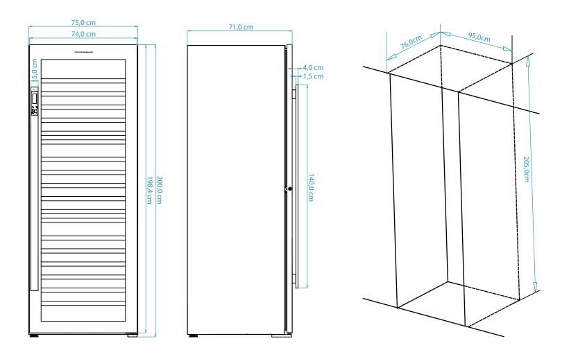
This model is designed for free-standing installation. Built-in installation is possible if the wine cooler has at least 5cm space on each side (like the above drawing). The air should be able to move freely in the space around the wine cooler.
